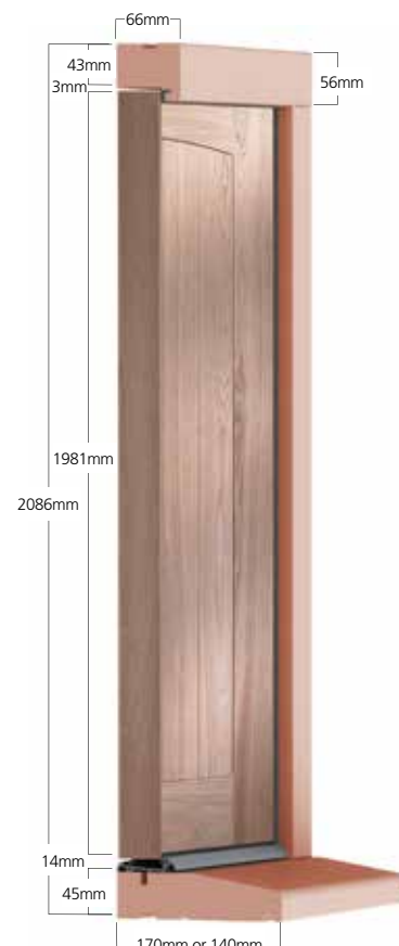
Vertical section of door frame (Diagram shown not to scale).
